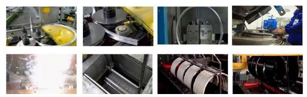
**Spokes-** First the procured and QC wire will be unrolled and straightened using a straightening machine. The wire is then fed through three sets of rollers to untwist it and is then cut, forming a spoke blank. Then the processes start to diverge. The wire is fed straight into the spoke-making machines and a speedy spoke a second comes out at the other end. Swaging is the process of cold forging the spokes to reduce the diameter.
