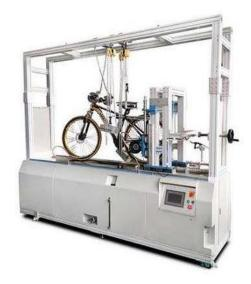
Wheels testing machine- This machine is used to measure Wheel dimension, Hub length, Rim edge width, etc.
